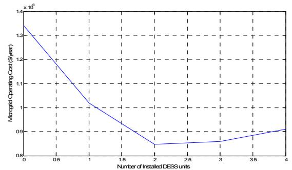
Figure 4. Microgrid operating cost with different number of installed DESS
