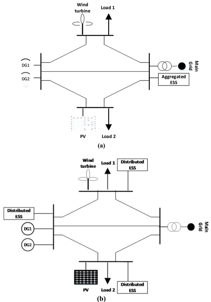
Figure 1. Integrating ESSs in the microgrid; (a) Aggregated, (b) Distributed .
