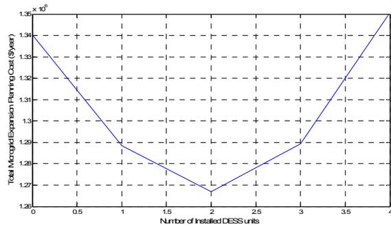
Figure 5. Microgrid total expansion planning cost with different number of installed DESS units
