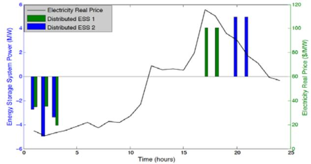
Figure 2. The charging/discharging power of DESS units and the electricity price for one sample day.
